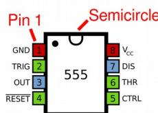
The NE555 timer chip should now be soldered in its space at the centre of the board. Pin 1 should be identified by a semicircular recess in one end of its plastic package, with the semicircle at the top pin 1 will be on the left. The PCB has an outline of IC1 with a semicircle printed on it, this should be aligned with the semicircle on the package.
