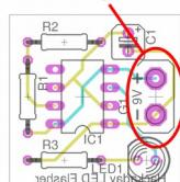
The battery connector is a plastic clip to fit a PP3 style 9v battery, with a red wire and a black wire to connect to the PCB. The ends of the wires should already have had their insulation removed, so you can solder them directly to the board. The red wire should go to the hole marked with a + symbol while the black wire should go to one marked with a -.
