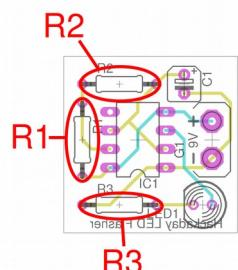
The LED cathode is identified by a shorter wire and a flat spot on the LED rim that corresponds with a flat on its outline printed on the board. The cathode wire should go in the hole closest to R3 on the board.
